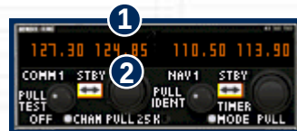
1-Standby frequency, 2-Standby flip/flop switch
