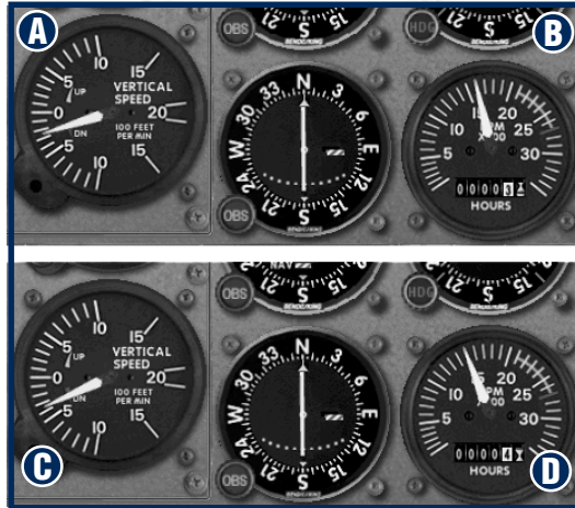
Figure 6-4 A-VSI and B-tachometer with slightly more power. C-VSI and D-tachometer with slightly less power
